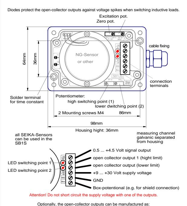
Optionally, the open-collector outputs can be manufactured as: upon exceeding trigger threshold conducting - version L or: upon exceeding trigger threshold non-conducting - version N
