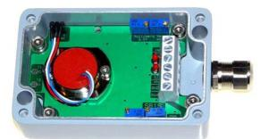
Sensor box containing one sensor, one signal conditioner with 0...5V output and two open-collector output switches
