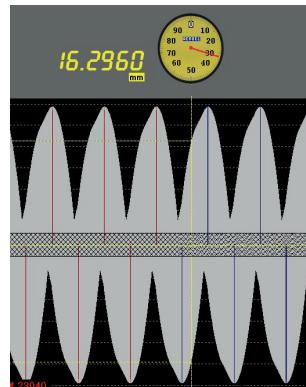
Using a special guided procedure, the operator seeks the starting point, moves the part to the measurement position and starts the measuring cycle: the part is rotated by a special motor driven device using a rubber wheel laying on the part. This keeps it pushed against the V blocks and assures a "zero run-out" rotation, that is a rotation around a perfectly fixed axis.
