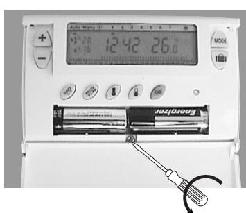
**ADJUSTMENT OPTIONS** You may choose to put on or not the anti-lock system of the circulation pump (see device's back face when it is removed)
