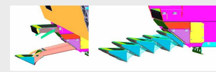
**THE IFE** TRACK ACCESS DEVICE facilitates the access of train drivers, adding a third step. It eases the entrance from track level especially in extreme weather conditions.
